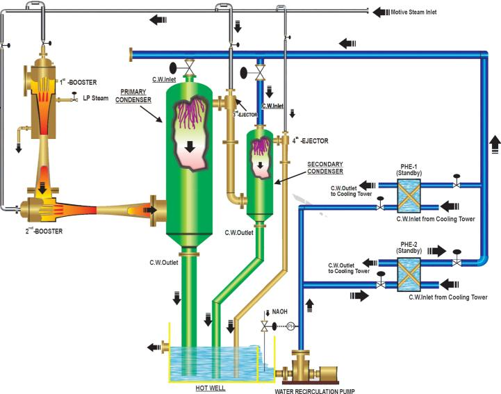
When the Closed Loop water circulation system is provided as shown in fig and it re-curculating and cool through the plate type heat exchanger the crystallizing fatty acid is despite on plate it resulted exchanger is fouling fastest. To avoid this problem sodium hydroxide solution is added. In this type of system additional condensate of motive steam, striping steam, separate though the special designed Hot-well and removing the additional liquid through over flow nozzle.
