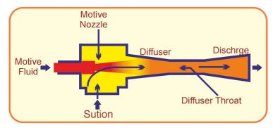
The Steam nozzle discharges a high velocity jet across the suction chamber. This steam jet creates a vacuum which extracts air or gas from the adjoining vessel. As these gases are entrained in the steam, the mixtures travel through the ejector in to a venture shaped diffuser. In the diffuser, its velocity energy is
